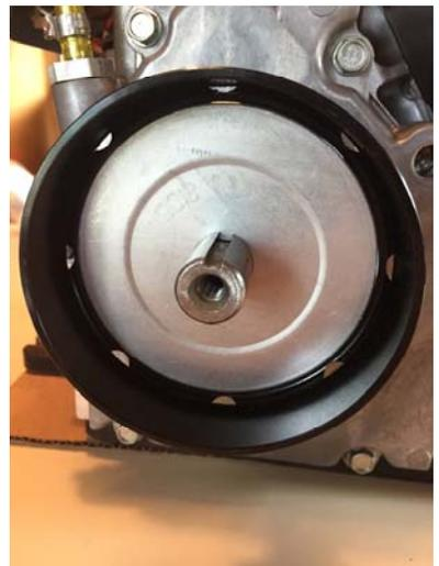
**Install the spring/shoe retaining washer.**
