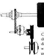
Chain Drive through differential with reverse gear box.
