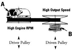
As the speed increases, the centrifugally actuated roller weights (A) follow the contour of the bowl-shaped ramp plate, forcing the driver sheaves together. this action through the belt compresses the driven-pulley spring (B), thus achieving a "high gear" ratio.
